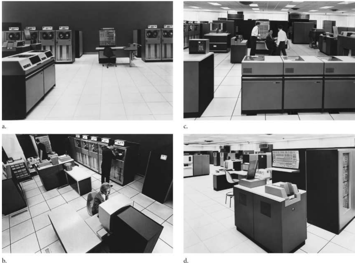
FIGURE e1.12.3 IBM System/360 computers: models 40, 50, 65, and 75 were all introduced in 1964. These four models varied in cost and performance by a factor of almost 10; it grows to 25 if we include models 20 and 30 (not shown). The clock rate, range of memory sizes, and approximate price for only the processor and memory of average size: (a) model 40, 1.6 MHz, 32 KB–256 KB, $225,000; (b) model 50, 2.0 MHz, 128 KB–256 KB, $550,000; (c) model 65, 5.0 MHz, 256 KB–1 MB, $1,200,000; and (d) model 75, 5.1 MHz, 256 KB–1 MB, $1,900,000. Adding I/O devices typically increased the price by factors of 1.8 to 3.5, with higher factors for cheaper models.
