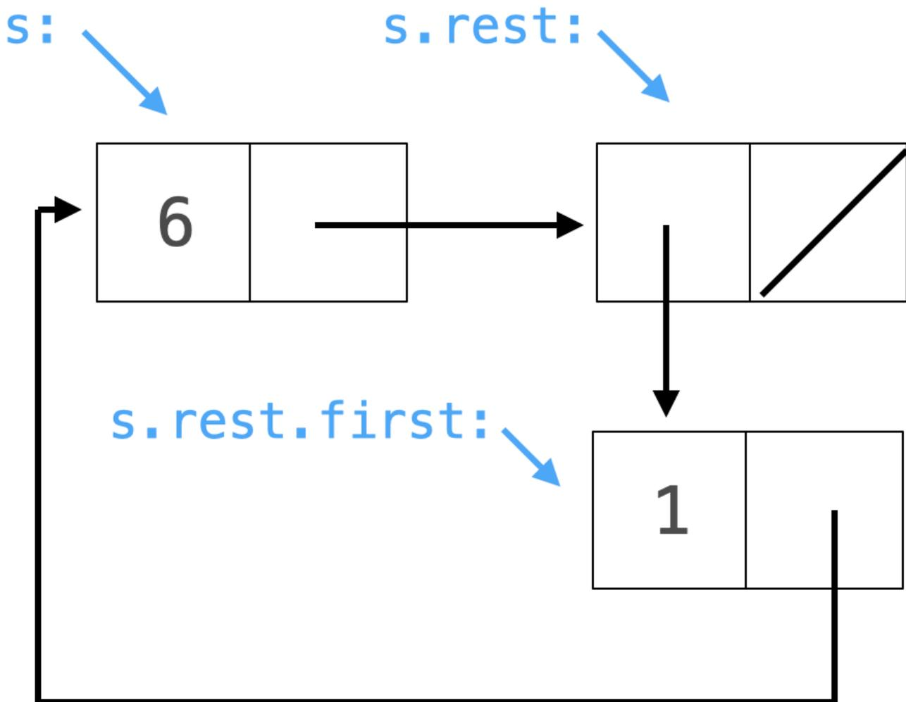
Making a cycle requires two steps: making a linked list without a cycle, then modifying it. First create, for example, `s = Link(6, Link(Link(1)))`, then change `s.rest.first.rest` to create the cycle.
