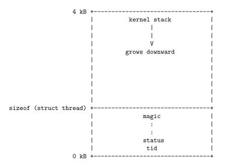
This layout has two consequences. First, struct thread must not be allowed to grow too big. If it does, then there will not be enough room for the kernel stack. The base struct thread is only a few bytes in size. It probably should stay well under 1 kB.
