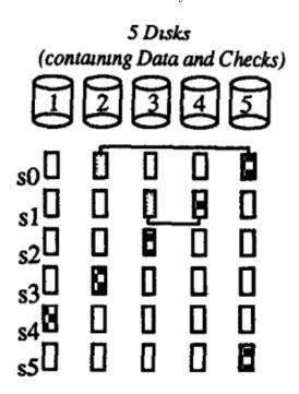
Note: Due to the large size of disks in practice, RAID V is no longer used in practice, because it is too likely that a second disk will fail while the first is recovering. RAID VI is usually combined with other error recovery techniques in practice.
