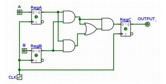
The maximum allowable hold time for RegC is how long it takes for RegC's input to change, so (clk-to-q of A or B) + shortest CL time = 4 + (5 + 5) = 14 ns.
