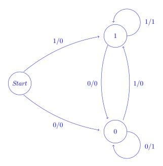
$\overline{5.3}$  Write an FSM that will output a 1 if it recognizes the regex pattern  $\{10+1\}$ .
