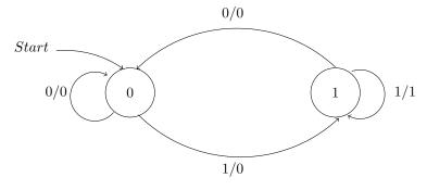
The FSM outputs a 1 if it detects the pattern "11". The FSM would output "001000000110"
