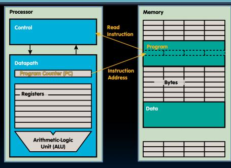
PC (program counter) is a register internal to the processor that holds <u>byte</u> address of next instruction to be executed
