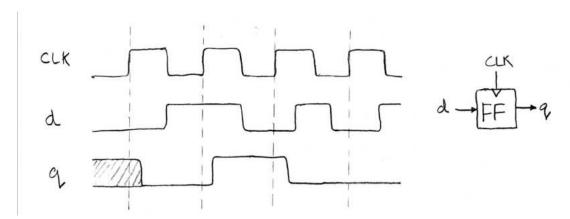
On each positive clock edge \_\_\_\_\_, the q output is changed to the current value of the d input.
