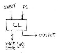
Given that we want to force a state transition on each clock cycle (remember inputs bits are being applied one per clock cycle), we will put the combinational logic block in a loop with the state register as shown below:
