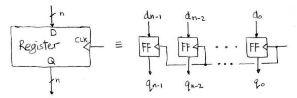
Here we are going to talk about the most common type of flip-flop, called an *edge-triggered d-type flip-flop*. Internally each flip-flop comprises around 10 transistors. The operation of the flip-flop is illustrated below. The illustration depicts the operation of one of two types of edge-triggered d-type flip-flops, a *positive* edge-triggered one (*negative* edge-triggered is the other). For the most part we will stick with positive edge flip-flops this semester.
