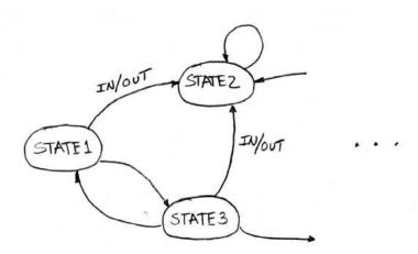
Given combinational logic circuits and registers, FSM, can be implemented in hardware.
