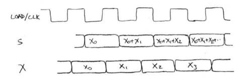
Later we will discuss the detailed timing of the operations in the accumulator circuit, but first we need to look at the detailed operation of the register.
