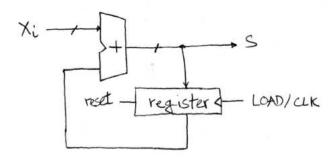
The register holds the current value of S while the next one is being formed. After we are happy with the next S, we load it into the register and apply the new X value, then wait for a new S to appear at the output of the adder. The process is repeated for all n X values.
