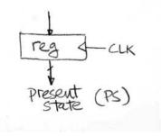
Now we need a circuit that implements a function that maps the input and present state to the next state and output. Because this circuit doesn't need to remember anything on its own, we can use a combinational logic circuit for this task.
