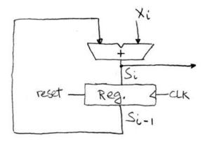
The output of the circuit is labeled  $S_i$ , and the output of the register is labeled  $S_{i-1}$  to remind us that the register delays the signal for 1 cycle. So if the output of the circuit is holding the result of the  $i^{th}$  iteration, then the register holds the result of the  $i^{th} - 1$  iteration.
