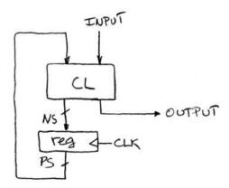
On each clock cycle the CL block looks at the input value and the present state and produces the bit pattern for the next state and generates an output of 0 or 1. On the rising edge of the clock the new state value get captured by the register and the process starts again.
