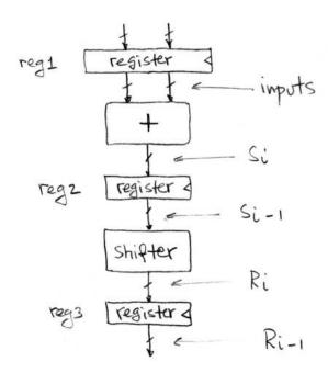
On each cycle, data moves from the output of reg1 through the adder to the input of reg2, or moves from the output of reg2 through the shifter to the input of reg3. Since no longer does the data need to move through both blocks on each cycle, the clock frequency can be increased. See the waveforms below:
